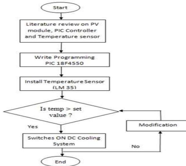
Fig. 2 Flow chart of the PIC controller system.
