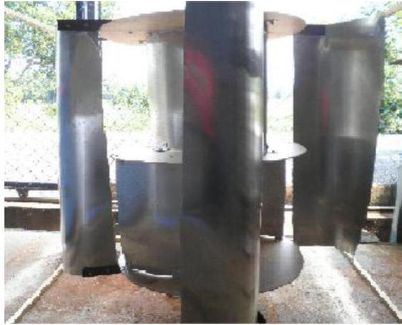
Fig. 6. Hybrid wind turbine of Savonius and Darrieus
