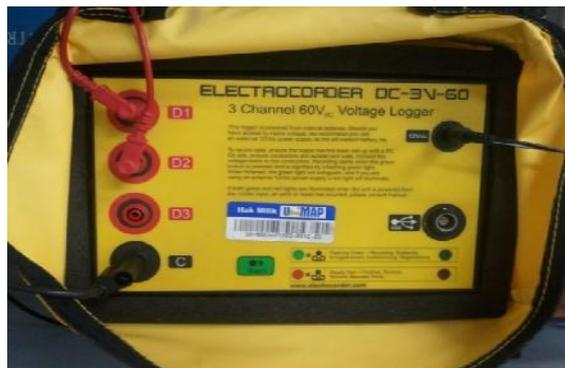
Fig. 4. Electrocoder for output voltage measurement
