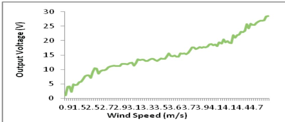
Fig. 11. The graph of output voltage from vertical axis hybrid wind turbine
