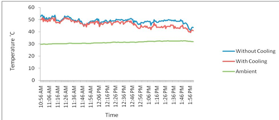
Fig. 9. Comparison between ambient temperature and average panel temperature under cooling and without cooling condition.
