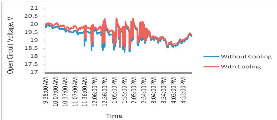
Fig. 10. The graph of the open circuit voltage under cooling and without cooling condition.
