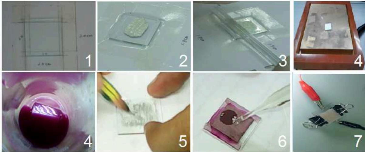
Fig. 3 Process of fabricating DSSC
