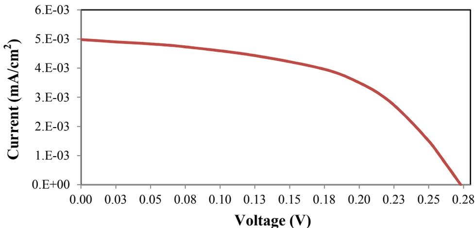
Fig. 5 Current-voltage curve for DSSC using Pitaya dye
