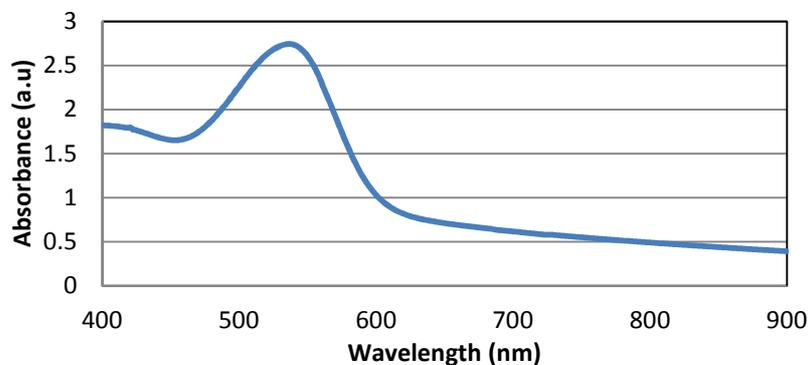
Fig. 4 UV-Vis Absorption spectra of Pitaya fruit's dye
