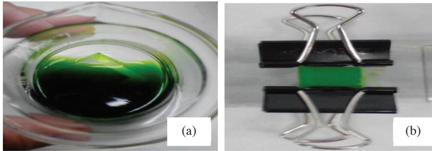
Fig. 3. (a) TiO<sub>2</sub> film is immersed into spinach's dye (b) Solar cell with chlorophyll dye
