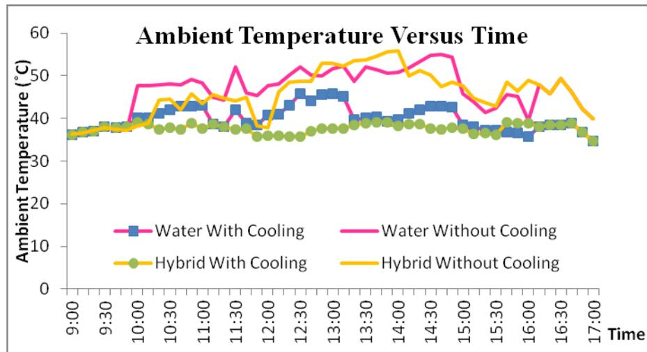
Fig. 2 Comparison of ambient temperature versus time between DC water pump and DC hybrid.
