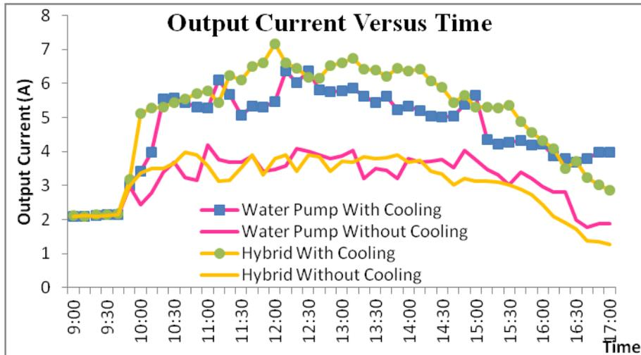
Fig. 4 Comparison of output current versus time between DC water pump and DC hybrid.
