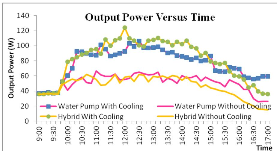
Fig. 5 Comparison of output power versus time between DC water pump and DC hybrid.
