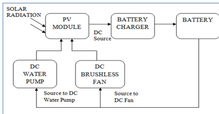
Fig.1 Block diagram overview of the investigation.
