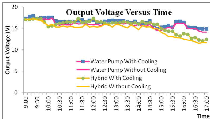
Fig.3 Comparison of output voltage versus time between DC water pump and DC hybrid.
