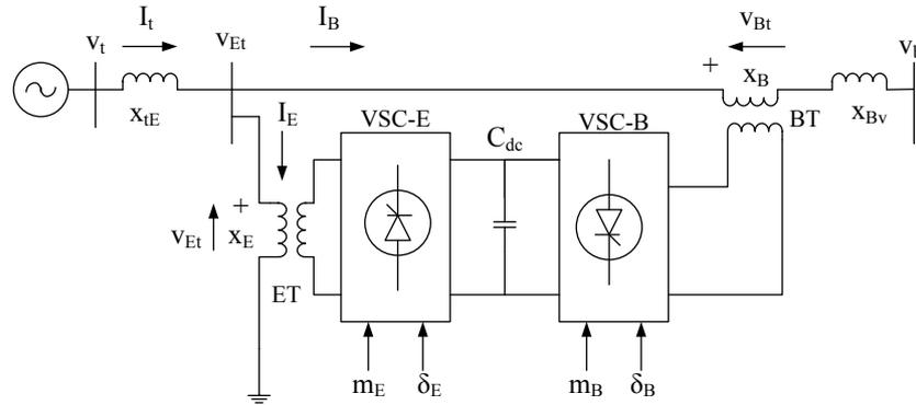
Figure 1: UPFC installed in single machine infinite bus power system
