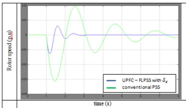
Figure 4: Change of rotor speed using damping controller  $\delta_E$
