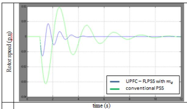
Figure 2: Change of rotor speed using damping controller  $m_E$
