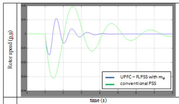
Figure 3: Change of rotor speed using damping controller  $m_B$
