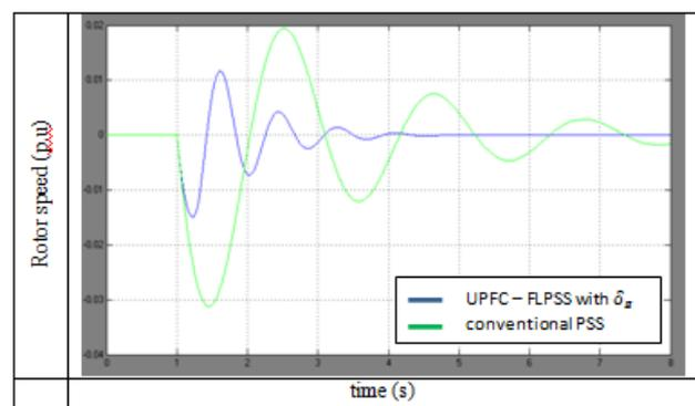
Figure 5: Change of rotor speed using damping controller  $\delta_B$
