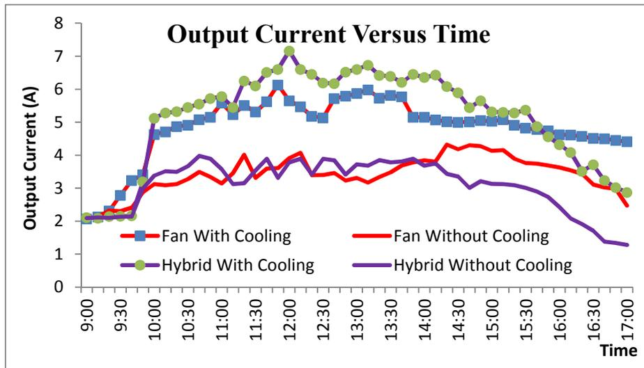
Fig. 4 Comparison of output current versus time between DC brushless fan and DC hybrid.
