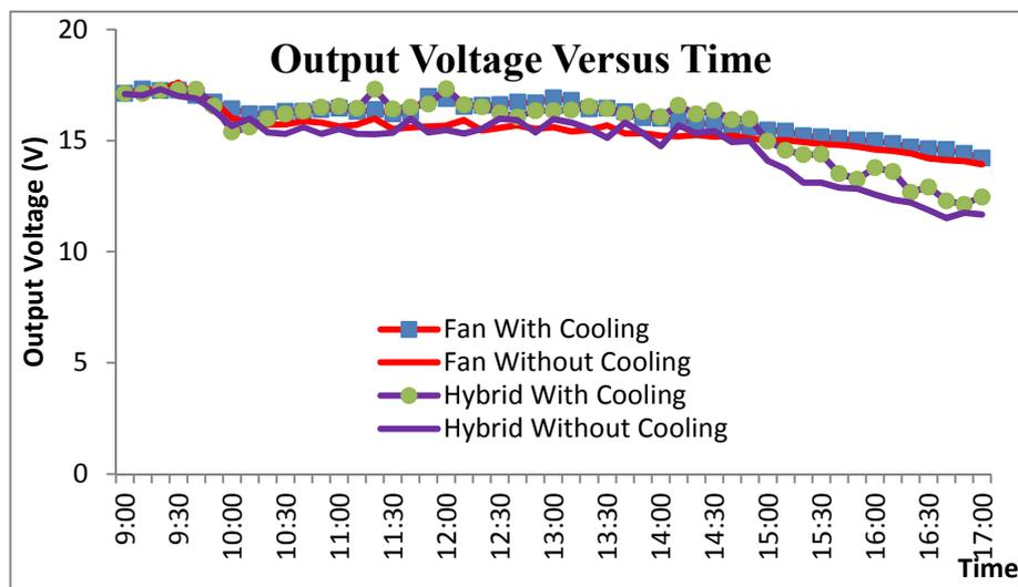
Fig.3 Comparison of output voltage versus time between DC brushless fan and DC hybrid.
