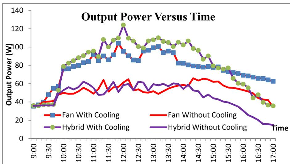
Fig. 5 Comparison of output power versus time between DC brushless fan and DC hybrid.
