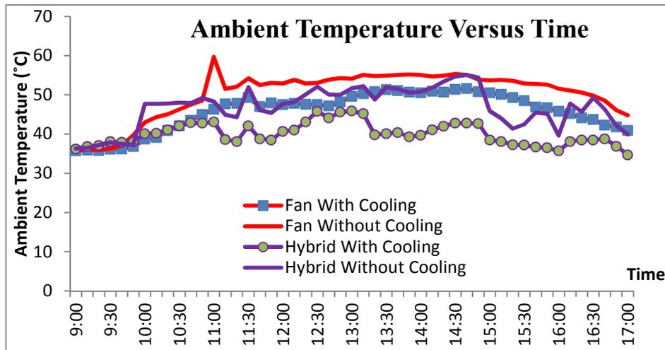
Fig. 2 Comparison of ambient temperature versus time between DC brushless fan and DC hybrid.
