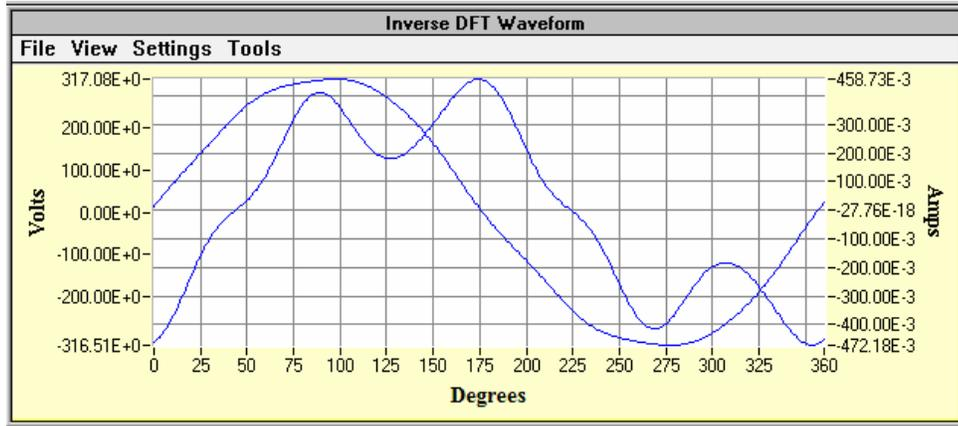
Fig. 5. Voltage and current waveform of loads
