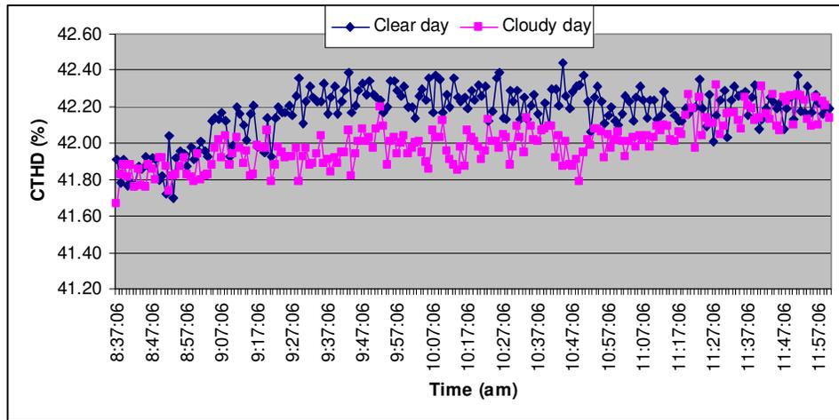
Fig. 7. Current total harmonic distortion
