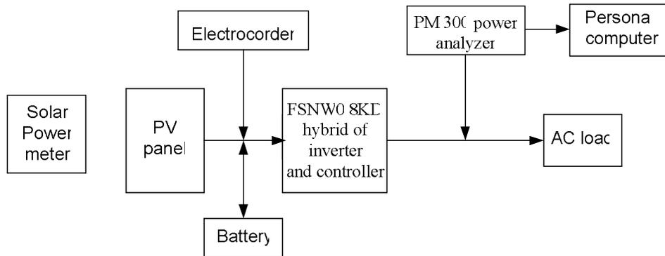
Fig. 1. Equipments block diagram
