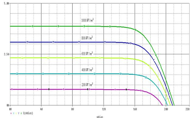
**Figure 3.** Current-voltage curve of PV module with  $200 \text{ W/m}^2$ ,  $400 \text{ W/m}^2$ ,  $600 \text{ W/m}^2$ ,  $800 \text{ W/m}^2$ ,  $1000 \text{ W/m}^2$  of solar irradiance and  $25^\circ\text{C}$  of constant temperature
