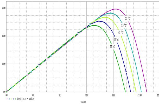
**Figure 6.** Power-voltage curve of PV module under  $1000 \text{ W/m}^2$  of constant solar irradiance and difference temperature
