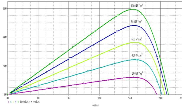
**Figure 4.** Power-voltage curve of PV module with 200 W/m<sup>2</sup>, 400 W/m<sup>2</sup>, 600 W/m<sup>2</sup>, 800 W/m<sup>2</sup>, 1000 W/m<sup>2</sup> of solar irradiance and 25 °C of constant temperature
