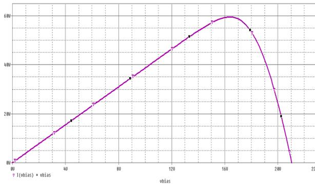
**Figure 2.** Power-voltage curve of PV module
