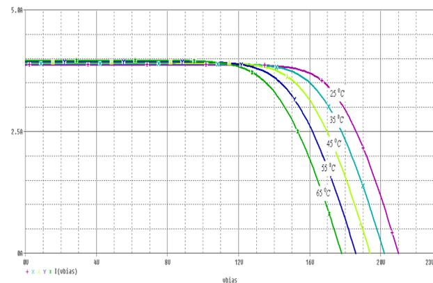
**Figure 5.** Current-voltage curve of PV module under 1000 W/m<sup>2</sup> of constant solar irradiance and difference temperature
