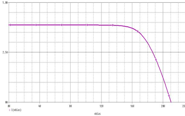
**Figure 1.** Current-voltage curve of PV module
