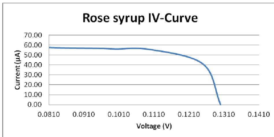
Fig. 5 Current-voltage for curve for DSSC using Rose's dye.
