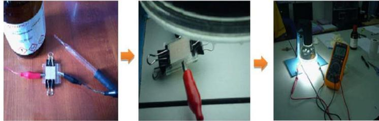
Figure 5 Indoor measurement by using halogen lamp
