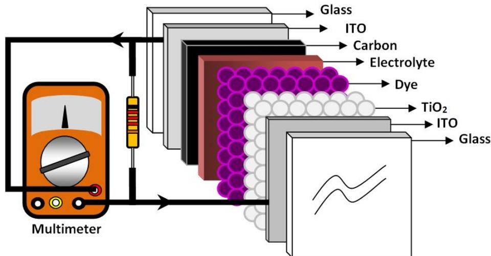
Figure 1 Schematic of the construction of Grätzel cell.
