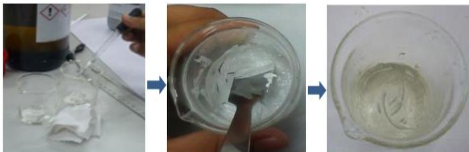
Figure 3 Preparation of TiO<sub>2</sub> Paste
