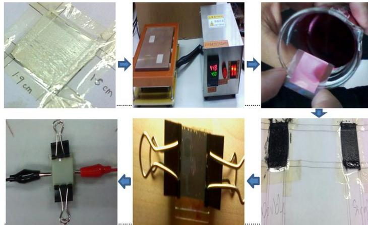
Figure 4 Steps of fabrication of DSSC using Dr. Blade
