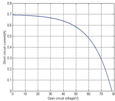
**FIGURE 8. I-V curve PV module at the temperature of 27.37 °C and Solar irradiance of 582.01 W/m<sup>2</sup>**
