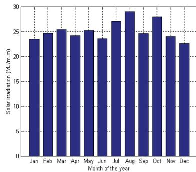
**FIGURE 3. Monthly estimated solar irradiation in MJ/m<sup>2</sup>**
