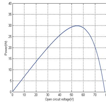
**FIGURE 9. P-V curve PV module at the temperature of 27.37 °C and Solar irradiance of 582.01 W/m<sup>2</sup>**
