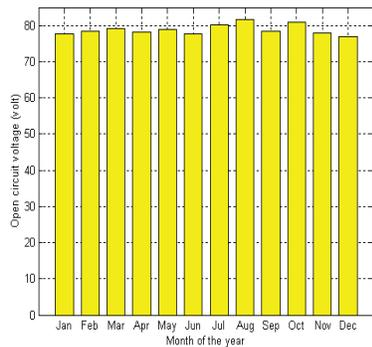
**FIGURE 6. Monthly open circuit voltage of PV module**
