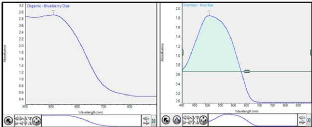
Fig 4. UV-Visible absorption wavelength graph for blueberry dye and blue dye
