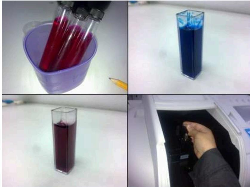
Fig 3. Blue and Blueberry dye tested in the Spectrometer Machine to obtain the Solar Absorbance reading
