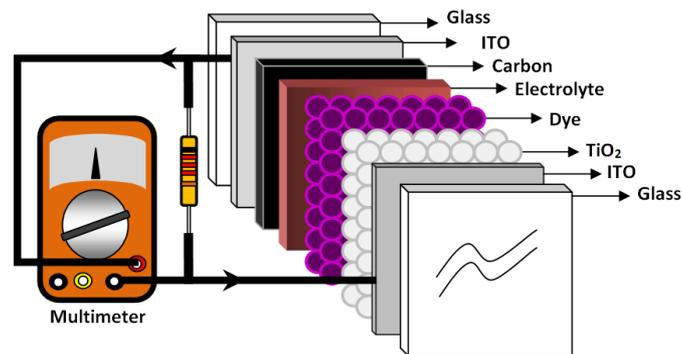
Fig 1. Dye Sensitized Solar Cell cross section
