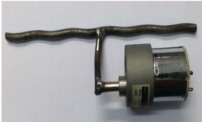
Fig. 3. DC Motor welded together with the shaft
