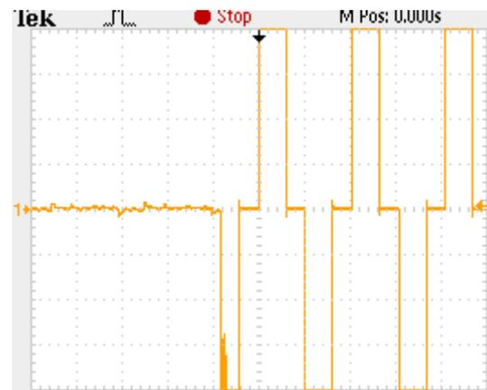
Fig. 12. Voltage wave form of proposed UPS inverter after the main source failure
