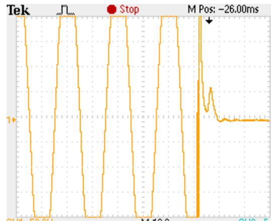
Fig. 11. Voltage wave form of main source failure
