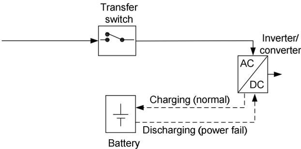
Fig. 3. Simplified block diagram of line interactive UPS
