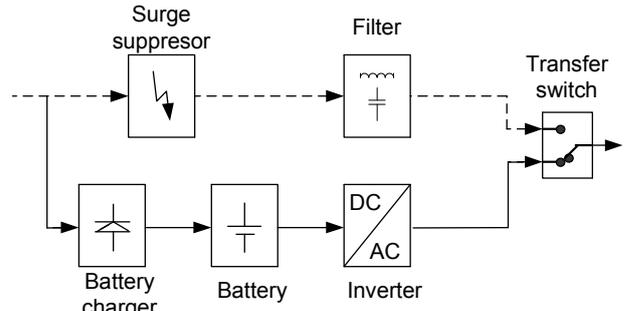
Fig. 4. Simplified block diagram of the online UPS
