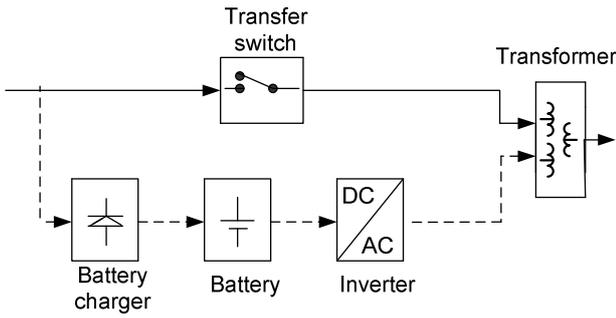
Fig. 2. Simplified block diagram of Ferroresonant UPS
