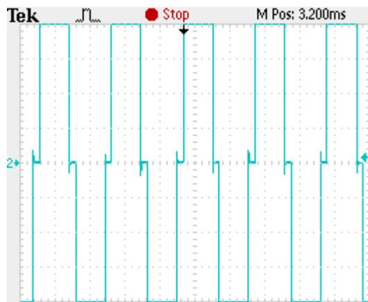
Fig.10. Experimental wave form of the voltage of the proposed UPS inverter
