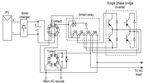
Fig. 5. A proposed circuit of photovoltaic powered uninterruptible power supply using smart relay
