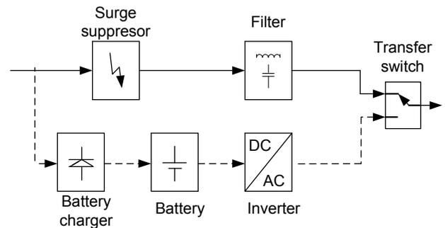
Fig. 1. Simplified block diagram of the standby UPS
