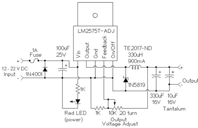
Fig. 6. Circuit of solar charger
