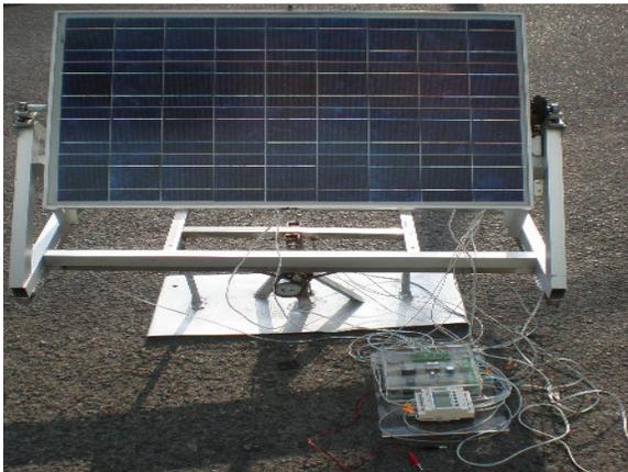
Fig. 3. A mechanic movement and input/output circuit of smart relay
