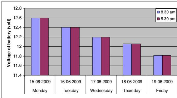
Figure 5. Battery was not charged
