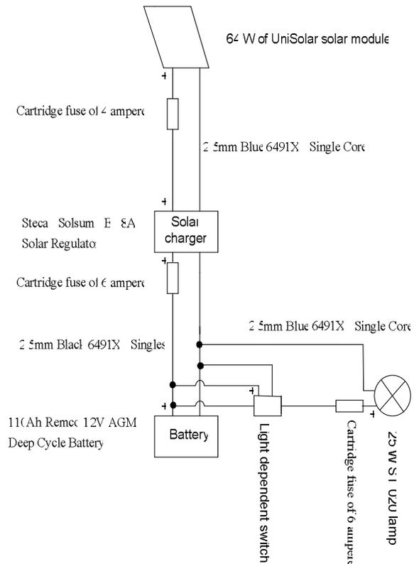
Figure 4. Wiring diagram for bulb of 25 W
