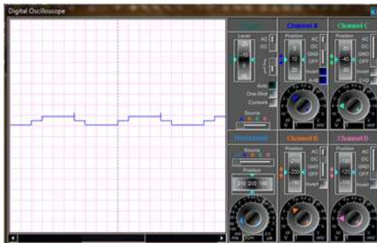
Figure 6: Three level AC output in Proteus software.
