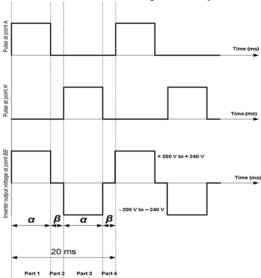
Figure 3: The duty cycle for PIC programmer.
