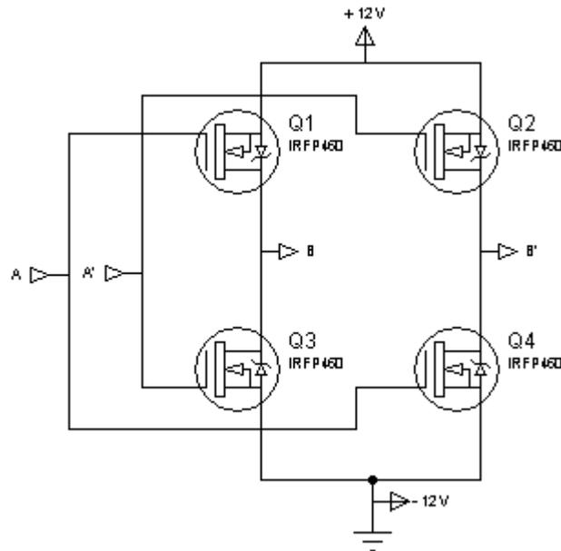
Figure 1: The Full bridge single phase inverter.
