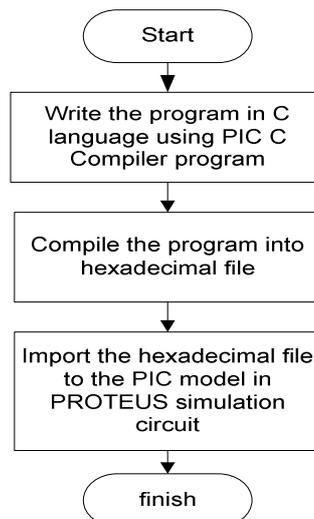
Figure 2: Flow chart of procedure to produce the AC three level voltage waveform.
