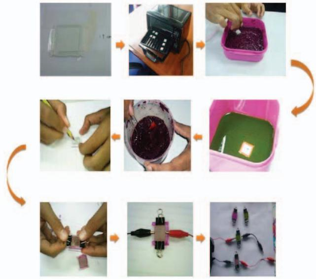
Fig 4. Steps of fabrication of DSSC
