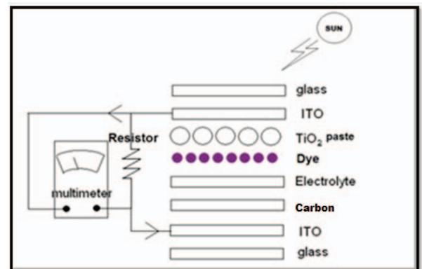
Fig. 1. Typical configuration of DSSC
