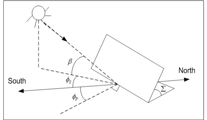
Fig 4: Illustrating the PV azimuth angle  $\phi_p$  and tilt angle  $\Sigma$  along with the solar azimuth angle  $\phi_s$  and altitude angle  $\beta$ . Azimuth angles are positive in the southeast direction and are negative in the southwest
