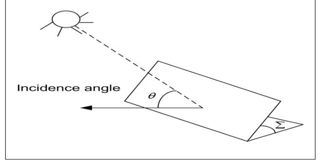
Fig 3: The incidence angle  $\theta$  between a normal to the PV module face and the incoming solar beam irradiance
