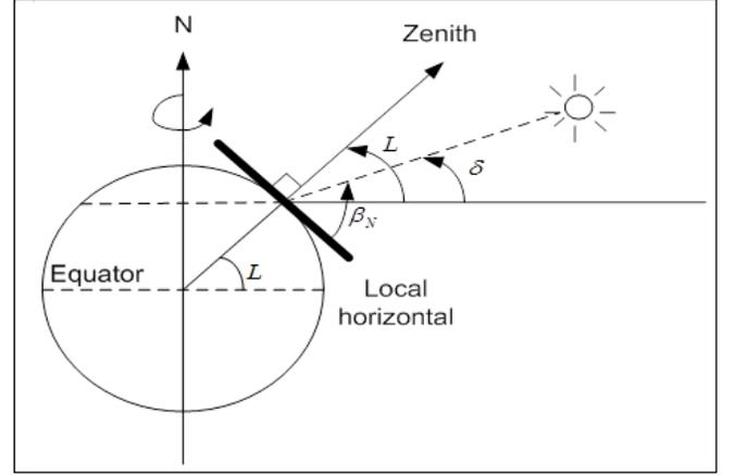
Fig 5: The altitude angle of the sun at solar noon
