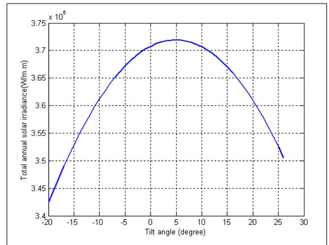
Fig 9: Annual total solar irradiance on different tilt angle of PV module
