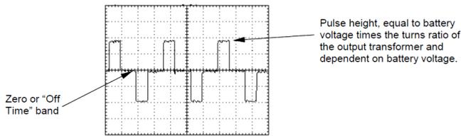
Figure 7. Modified Square Wave and Off Time.
