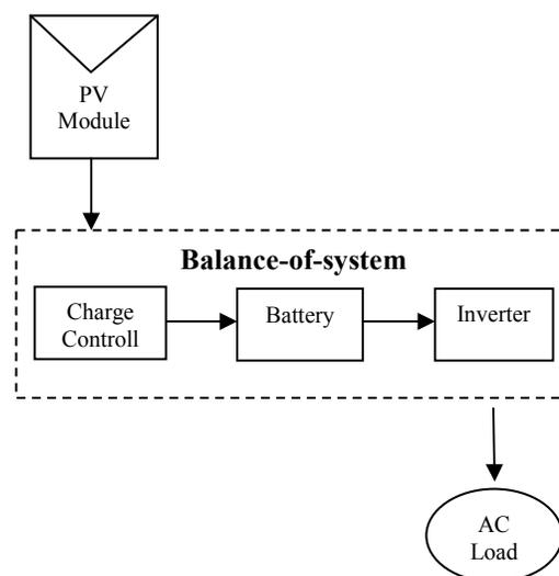
Figure 1. Block diagram representation of Photovoltaic System.
