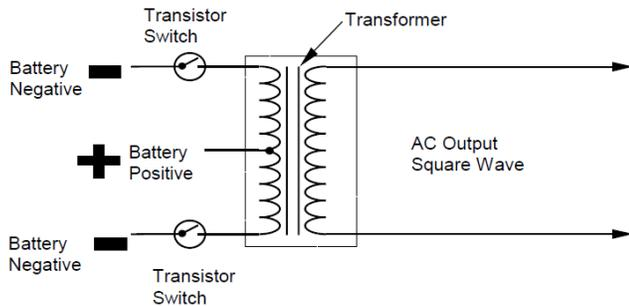
Figure 3. Push-Pull Topology for Square Wave Output.
