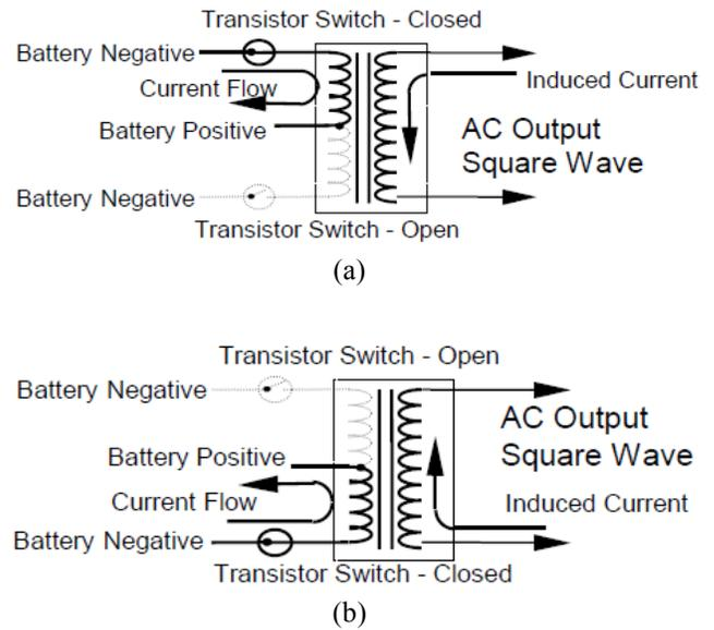
Figure 4. (a) Top switch close state, (b) Bottom switch close state.
