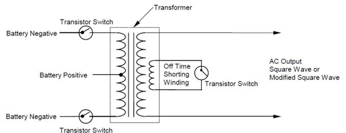
Figure 6. Push-Pull Topology with Shorting Winding.
