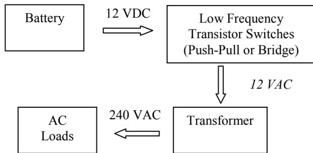
Figure 2. General flow of an inverter.
